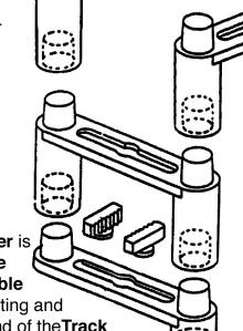
Note too, that the **Double Extender** can be mounted and rotated by using just **one** of its two **Columns!**Both columns dont need to be locked in.
