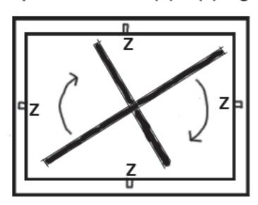
Step 2: Drop assembled Parts (E) & (F) into box as shown above. Then lift dividers up slightly and rotate until you are able to drop each panel (E & F) into their groove at points (Z) above.
